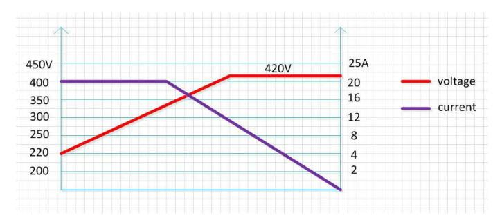
The charging current will be limited to ensure charger power will not exceed 6.6KW. The charge curve is an example under 230Vac input and 25°C ambient temperature. The charge curve will be different if different AC input current. The coolant and ambient temperature will also influence the charging power to ensure the internal components will not exceed its safe operation range.
